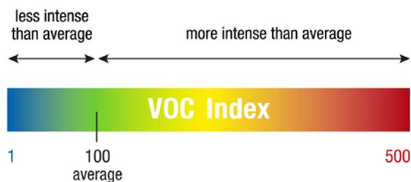
Figure 1 The indoor air quality can be monitored thanks to the VOC Index output of the SGP40 sensor.
