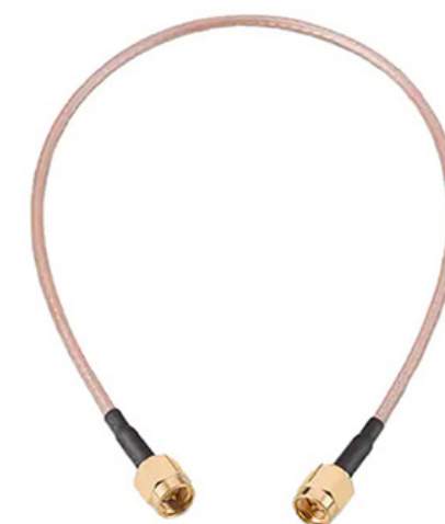
Figure 18: The 65503503530505 is a standard 12-inch coaxial cable assembly using RG-316 cable with straight SMA male plugs on each end; note the strain relief between connector and cable. (Image source: Würth Elektronik)
