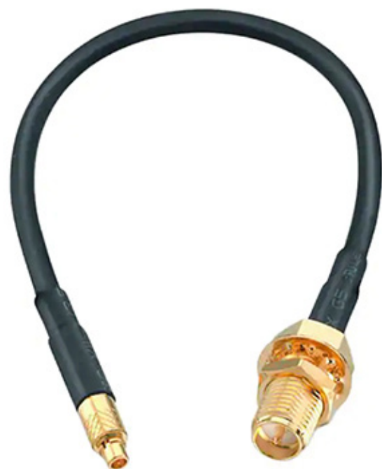
Figure 20: Cable assemblies can also be used as transitions between different connector families; the 65530260515303 assembly, for example, uses RG-174 cable and has an RP-SMA bulkhead male jack on one end and a straight MMCX male jack on the other. (Image source: Würth Elektronik)
