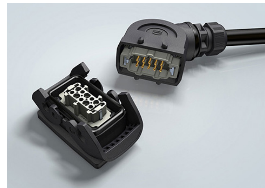
Figure 2: Han-series connectors (with four and 26 pins) are somewhat of an industry standard – satisfying various data and power-connectivity requirements from 50 to 5,000 V and 3 to 200 A. Locking arrangements include a single-lever Han-Easy Lock for easy single-handed operation and a double-lever Han-Easy Lock – for more reliable locking, higher pressure tightness, and use with cable-to-cable connections. Yet another rugged option is screw locking for maximum pressure tightness and reduced risk of unauthorized use. (Image source: Harting )
