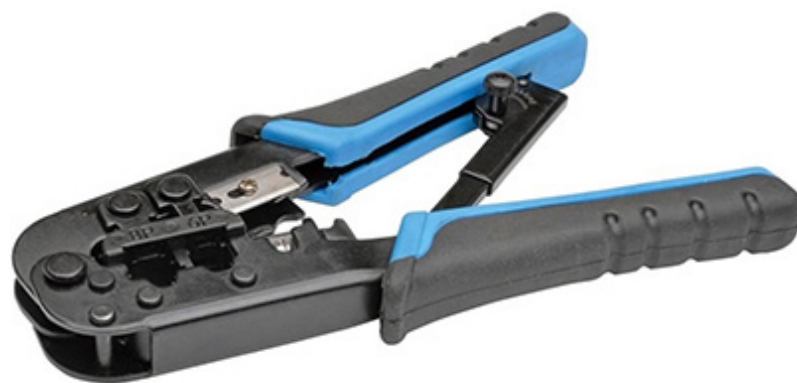
Figure 2: This is a TL2253-ND hand crimper tool that allows in-field RJ-plug termination of four, six, and eight-wire Ethernet cable cut to length. With one squeeze the tool's blades strip flat or round Cat5e and Cat6 and secure the connector body. (Image source: Tripp Lite )
