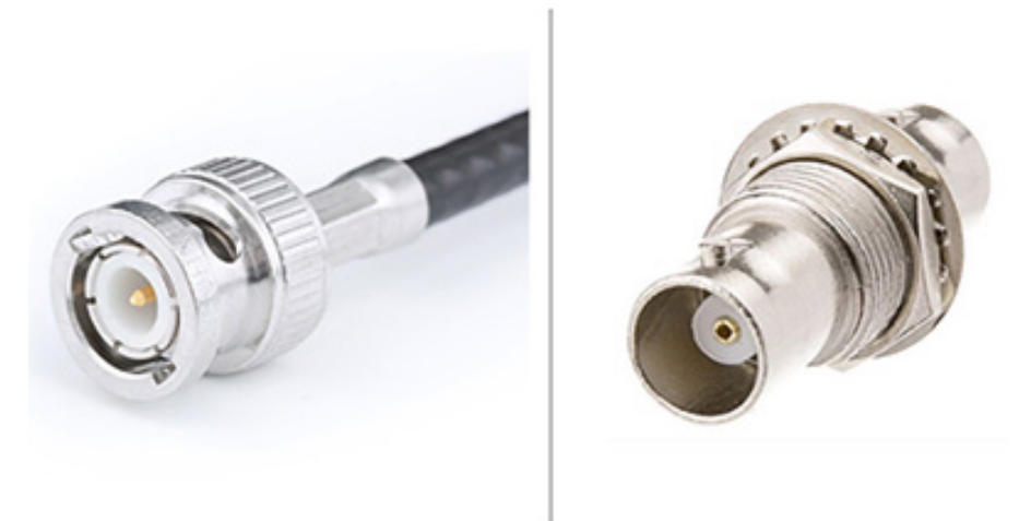
Figure 1: The BNC connector includes a bayonet body lock and has been widely used since its development in the early 1950s, but it is not a good electrical or mechanical fit for many of today's high-frequency, space-constrained applications. A male plug is usually used with cable assemblies (left); a female jack (right), for use on instrument panels. (Image source: Wikipedia; Pinterest)
