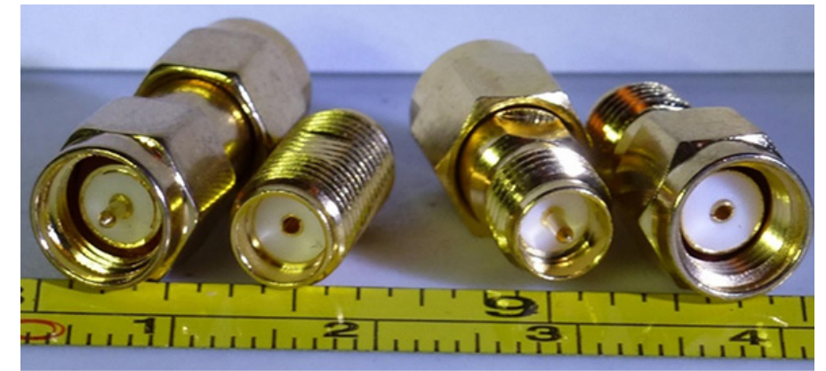
Figure 13: RP SMA plug and jack connectors have the opposite center conductor gender compared to conventional SMA connectors; (left to right) standard SMA male connector, SMA standard female connector, RP-SMA female connector, RP-SMA male connector. (Image source: Wikipedia)
