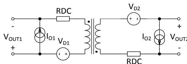
Figure 5: Primary and secondary voltage drops affect  $V_{OUT2}$
