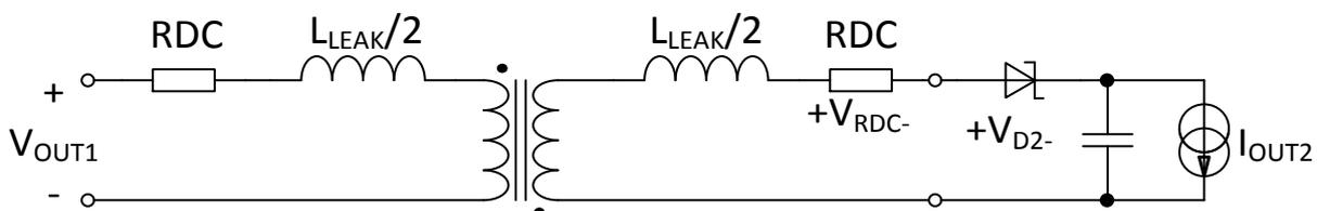
Figure 3: 1:1 Inductor with 1<sup>st</sup> Order Parasitic Components and Voltage Drops
