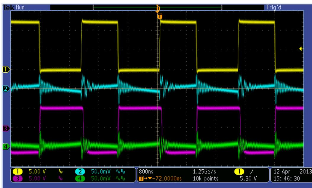
Figure 12: Steady State Waveforms.  $I_{o1} = 500 \text{ mA}$ ,  $I_{o2} = 100 \text{ mA}$
