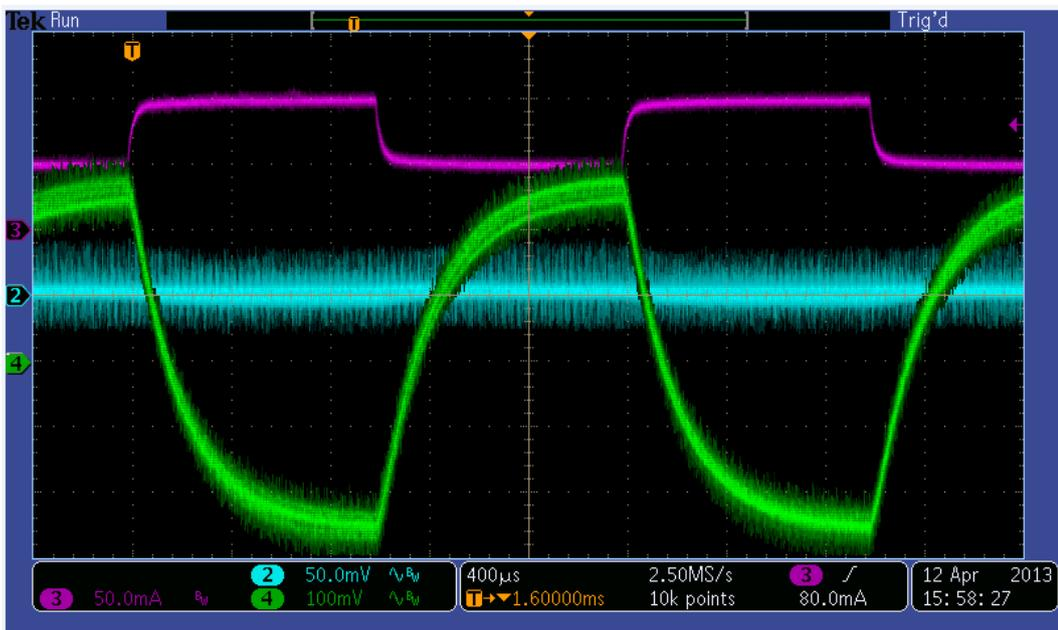
Figure 14: Load Transient on Secondary.  $I_{O1} = 500$  mA,  $I_{O2}$  varies from 50 to 100 mA
