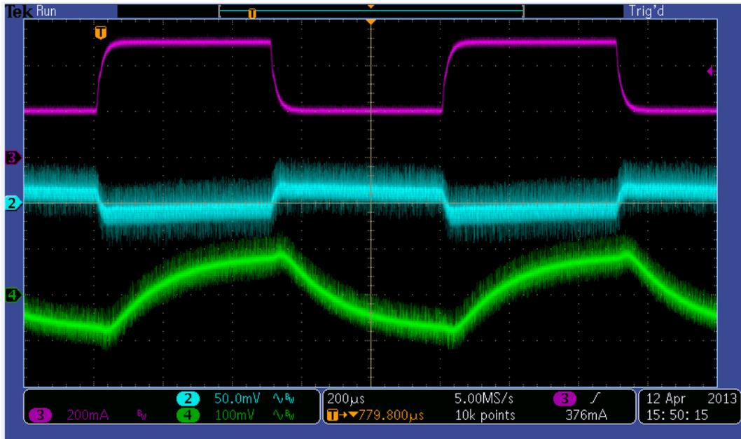
Figure 13: Load Transient on Primary.  $I_{O1}$  varies from 200 to 500 mA,  $I_{O2} = 100$  mA
