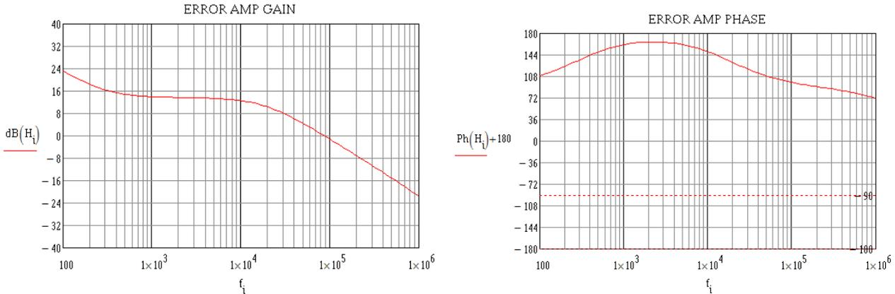
Figure 8: Error Amp Gain and Phase
